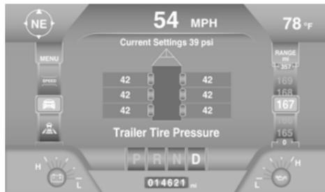
Trucks equipped with TTPMS will be delivered with four loose tire pressure sensors in the truck's cabin. These sensors must be installed in the desired trailer tires and then paired to the truck. Additional sensors can be purchased at an authorized Ram dealership.
